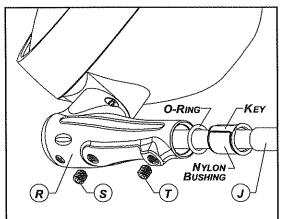
Fig. 2: Exploded View of Head Housing Assembly.
