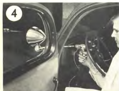
Press light through drilled hole—attach inside bracket, adjust frictions and the stop. Attach wire to ammeter. That's all there is to it!
