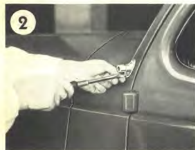
Position the bracket over the 1/8" drill holes and attach with self-threading screws.
