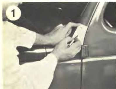
Position template enclosed with each bracket set in the manner shown above. Spot and drill two 1/8" holes.
